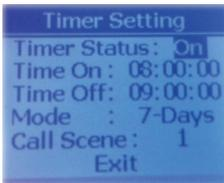
Timer setting is where the user can program Scenes to be triggered by the built in clock. The user has the ability to choose an already programmed scene and adjust when the cue will come on and turn off. A Max of 16 Timers can be set. The user can also choose from a variety of Modes within Timer Setting. The Mode contains the following options:
