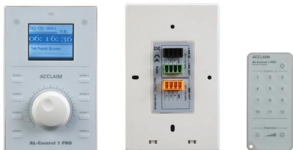
The **AL-Control 1 Pro** is a professional, multi-function DMX controller, designed for RGB LED fixtures. It features 12 programmable scenes, 7 built in effects and an internal time clock for triggering. Ambient light and proximity sensors allow the controller adapt to it's environment. It is a simple, yet powerful solution for wall mount DMX control.
