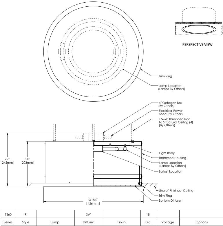
36 - 1 x 22 + 40 Watt SW - Satin White 19 - Painted Anodized U - 120-277 V DM - Specify Dimming Ballast R - Recessed 18" / 2GX13 **Opal Acrylic** Aluminum 1 - 120 V Consult The Factory 2 - 220-240 V EM - Fluorescent Emergency, 21 - Painted White 034 - 4 x 26 Watt 22 - Painted Custom 3 - 277 V Battery - Remote / GX24q-3 Color Other 174 - 4 x 24 Watt /2G11
