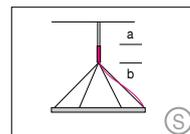
Suspension with pendant canopy PB 366 and steel cables
