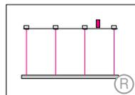
Suspension with current-carrying steel cables and cavity wall box. Not in connection with RGB.
