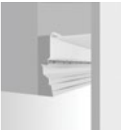
V Cove Perimeter wallwash with hidden source and knife edge detail for both gypsum and tile ceilings
