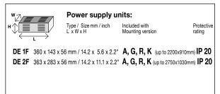
Input voltage for all external power supply units and canopy is 120-277 VAC 50-60 Hz
