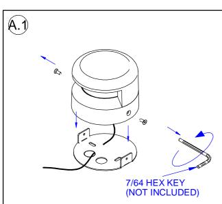
Remove the mounting bracket from the fixture.
