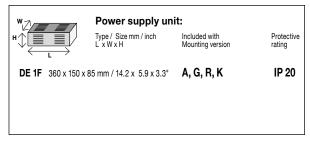
Input voltage for all external power supply units and canopy is 120-277 VAC 50-60 Hz
