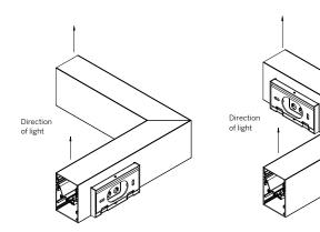
Mitered + Welded Housing Mitered + Butted Lens
