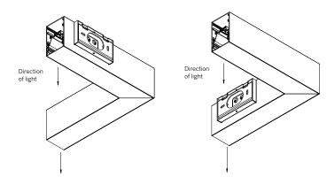
Mitered + Welded Housing Mitered + Butted Lens
