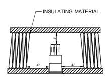
Recommended minimum distance from ceiling / insulating material
