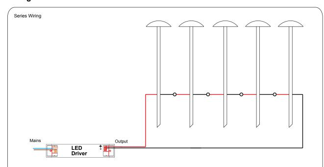
Note that while constant current light sources can be wired in series, the number of fittings that can be wired in series is limited by the forward voltage and wattage of the LED.
