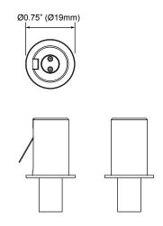
A  $\emptyset$ 0.75" ( $\emptyset$ 19mm) hole is required for mounting. Mounting surface min 0.2"(5mm)
