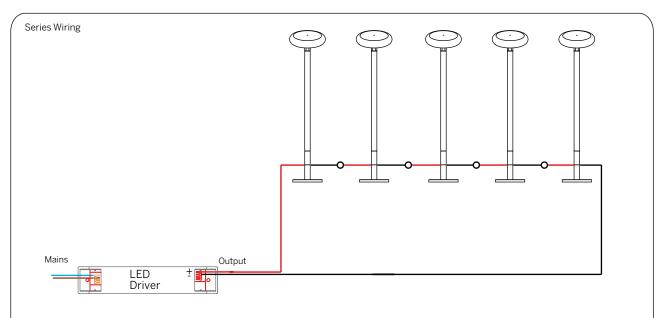
Note that while constant current light sources can be wired in series, the number of fittings that can be wired in series is limited by the forward voltage and wattage of the LED.
