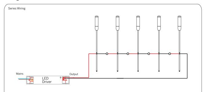
Note that while constant current light sources can be wired in series, the number of fittings that can be wired in series is limited by the forward voltage and wattage of the LED.
