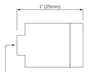
Fitting is secured via magnet (MAG) or via a suitable m3 fixing (SD)
