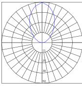
Beam Angle (0-180) = 71.6° Beam Angle (90-270) = 68.8°
